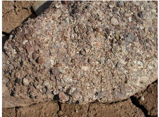
Figure 4. Polymict conglomerate characteristic of the sediment within the esplayed sandstone channels such as shown in Figure 3.
