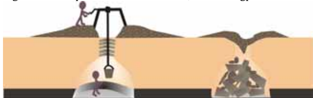
Figure 38. Diagram illustrating profile of a bell pit.
