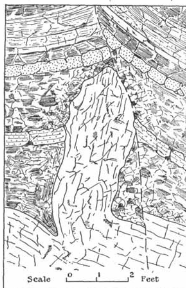
FIG. 2.—Titterstone Cleve, office quarry. Junction between the upper surface of the igneous sheet and the Coal Measures, with a tongue of basalt penetrating the overlying sediments, which are disturbed and altered.
