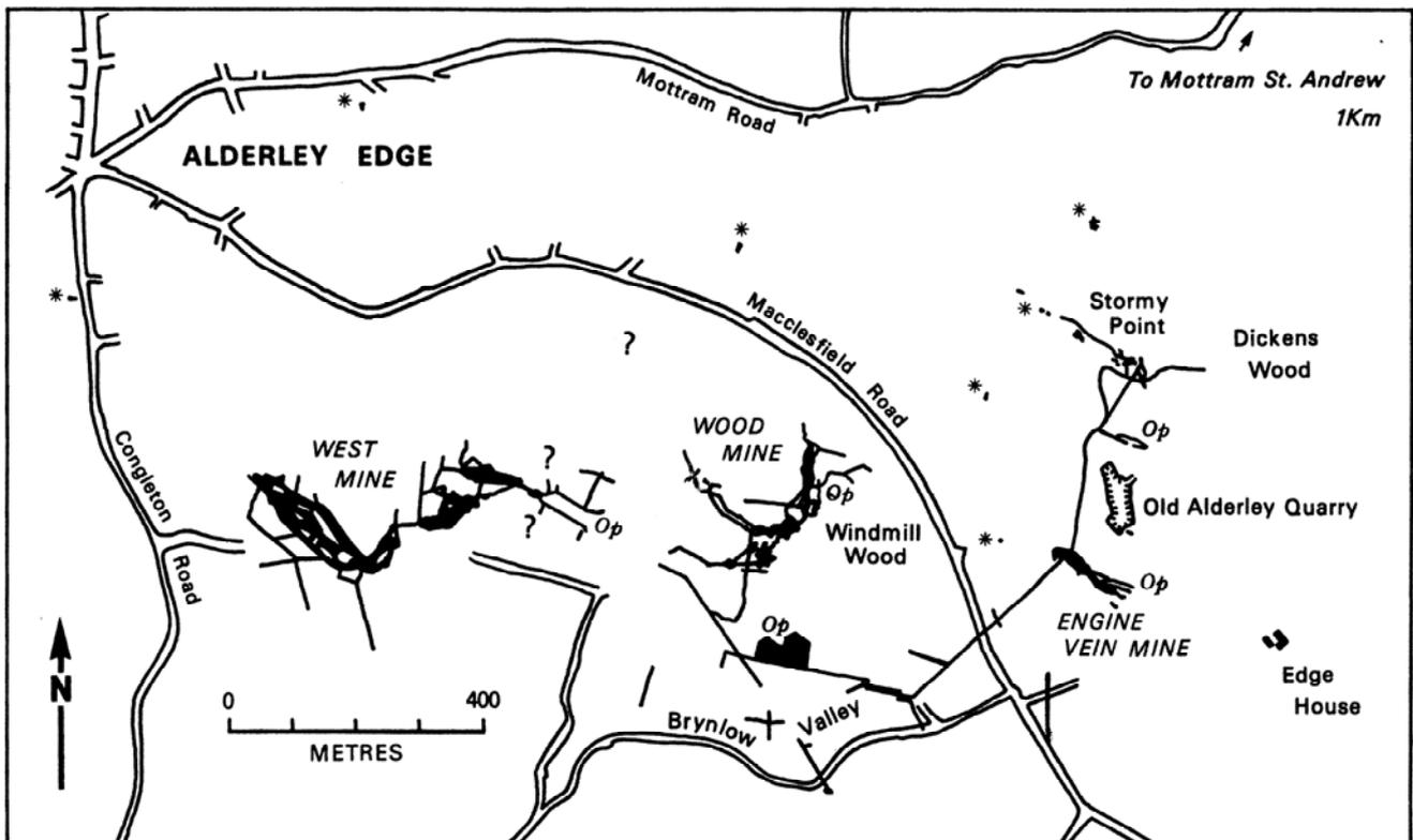
Figure 3. Distribution of mine workings at Alderley Edge (after Warrington, 1981, fig.2). Op – opencast workings (mostly infilled); \* – minor workings; ? – areas of possible workings.
