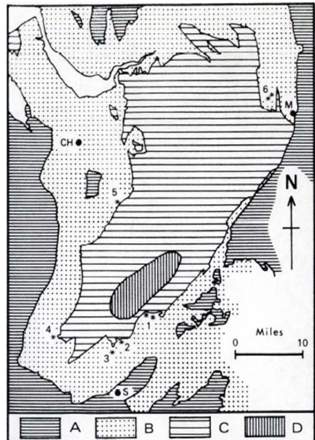
Figure 1. Locations of non-ferrous ore deposits in Triassic rocks in the Cheshire Basin (after Warrington, 1980b, map 1, in which the geology was based, with permission, on Institute of Geological Sciences 1: 625000 map, 3<sup>rd</sup> edition, solid, 1979).
