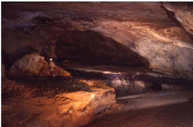
Figure 9. Part of a stope left after the extraction of a large body of copper ore hosted by aeolian sandstone, West Mine, Alderley Edge (photo: G. Warrington).
