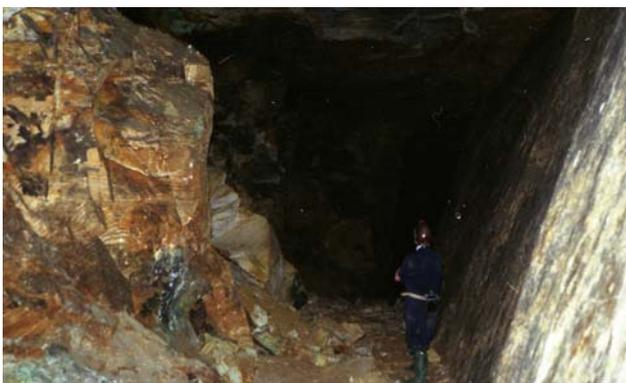
Figure 6. Upper level, Clive Mine, looking north; fault to the right of workings in the hanging wall (photo: G. Warrington).
